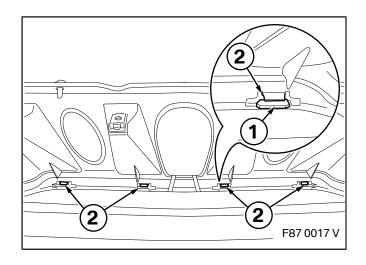
Removal of the standard rear diffuser insert as per ISTA.
