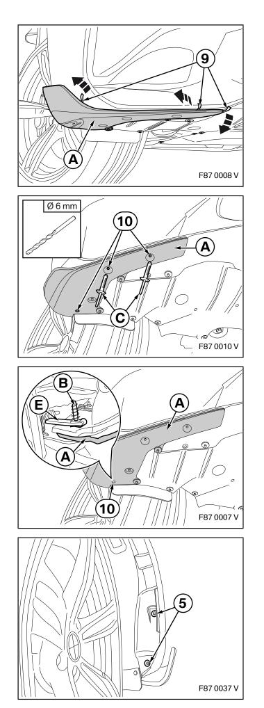
Remove the protective films (9) and press front addon **A repeatedly** and **firmly** onto the car.
