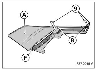
We recommend checking the fit of carbon front add-on section **A** on the car before applying the liquid adhesive and removing the adhesive backing films. During the later final assembly with liquid adhesive, sufficient space must be left between the front apron (3) and the top of carbon front add-on section **A**. ◀
