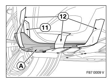
Clamp a suitable spacer (11) between carbon front add-on section  $\bf{A}$  and the front apron, then secure carbon front add-on section  $\bf{A}$  to the car using suitable adhesive tape (12).
