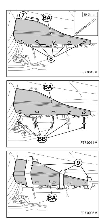
Clamp a suitable spacer (7) between carbon side skirt add-on section **BA** and the car. Drill five holes (8) from underneath with a **diameter of 6 mm**.
