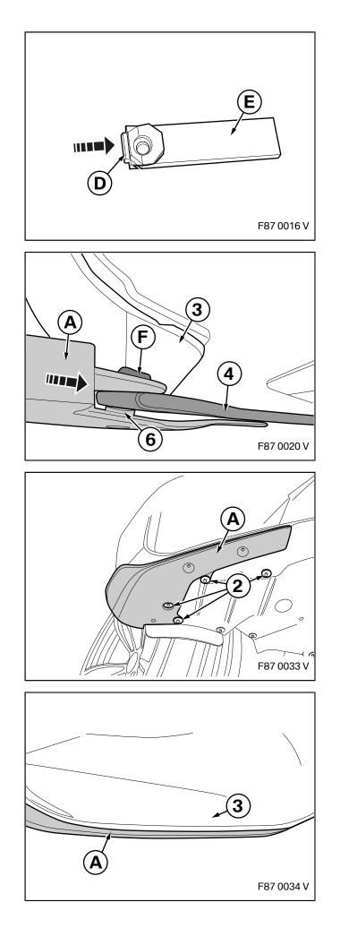
Attach C-clip **D** to plastic plate **E** as shown.
