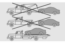
The vehicle should only be transported on a loading platform.
