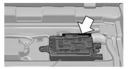
Information on the fuse types and locations, as well as the positions of any other fuse boxes, is found on a separate sheet in the fuse box.
