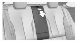
Press the switch and pull the center section forward.
