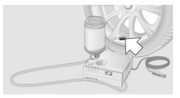
6. With the compressor switched off, insert the plug into the power socket inside the vehicle.
