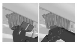
Extend the vehicle jack by turning the vehicle jack crank or lever clockwise.
