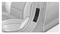
These tire inflation pressure values can also be found on the tire inflation pressure label on the driver's door pillar.
