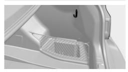
A multi-function hook is located on each side of the cargo area.
