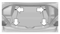
To secure the cargo there are two or four lashing eyes in the cargo area.
