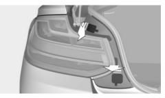
3. With the handle of the screwdriver from the onboard vehicle tool kit, loosen and remove the nuts on the two fasteners. Make sure that the nuts do not drop into the bumper area. In addition to the two outer fasteners, there is another inner fastener.
