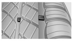
Wear indicators are distributed around the tire's circumference and have the legally required minimum height of 0.063 inches/1.6 mm.
