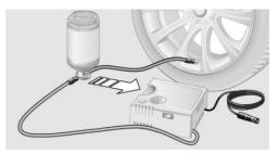
5. Remove the valve cap from the tire valve and screw the filling hose of the sealant container onto the tire valve of the nonworking wheel.
