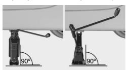
7. Crank up the vehicle jack until the entire surface of the jack is in contact with the ground and the wheel in question is raised a maximum of 1.2 inches/3 cm off the ground.
