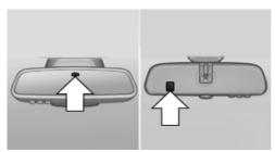
Photocells are used for control:
