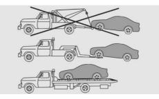
Your vehicle should be transported with a tow truck with a so-called lift bar or on a flat bed.
