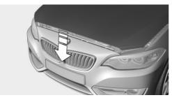
Let the hood drop from a height of approx. 16 inches/40 cm and push down on it to lock it fully. The hood must engage on both sides.
