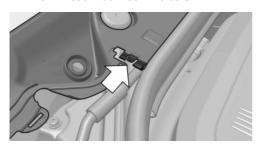
3. Press down on the holder and tighten the three screws.
