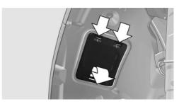
If necessary, pull the inside trim of the wheel house slightly inward. Turn the bulb socket counterclockwise and remove.
