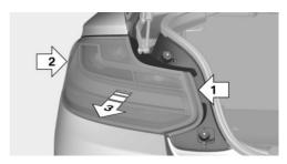
5. Remove the plug from the bulb holder.
