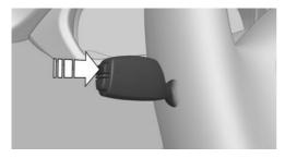
Press and hold button on signal lever.
