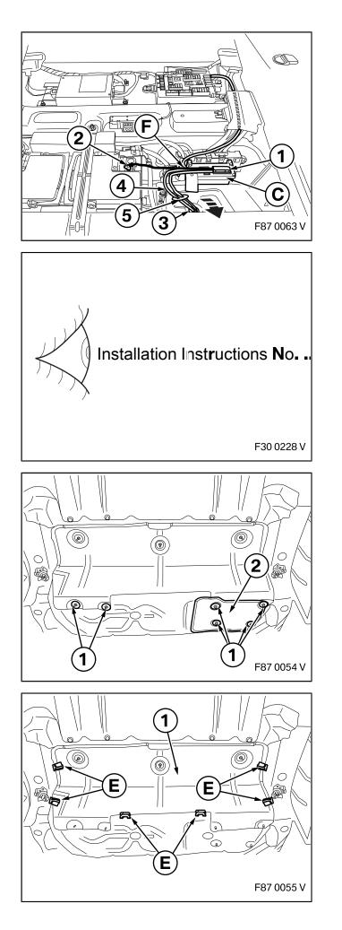
Insert the large plug on tailgate silencer wiring harness **F** into the large socket (1) on tailgate silencer receiver unit **C**. Screw the small cable to the earth post (2). Remove the sealing plug for the opening (3) from the boot tray. Thread the two tailpipe silencer plugs (4) through the opening (3) and attach the rubber bung (5) from tailpipe silencer wiring harness **F**.
