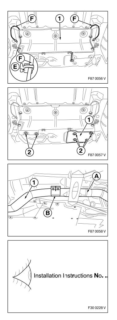
Route tailpipe silencer wiring harness **F** along the edge **above** the heat insulation (1) and secure it in the cable clips **E**.
