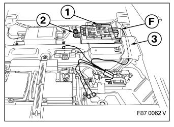
Screw tailgate silencer receiver unit **C** using both nuts (1) to the distributor (2) in the boot floor.
