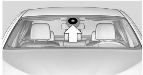
The camera is installed near the interior mirror. Keep the windshield in the area behind the interior mirror clean and clear.
