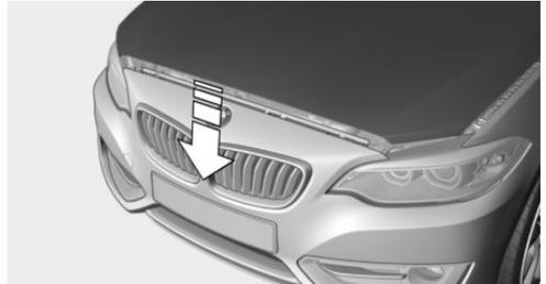
Let the hood drop from a height of approx. 16 inches/40 cm and push down on it to lock it fully.
