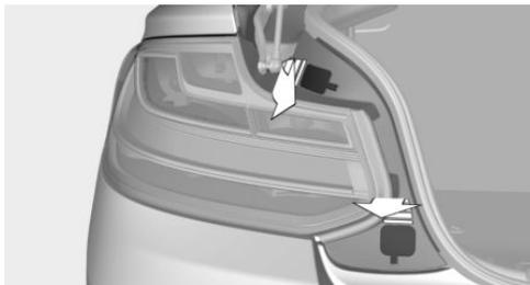
3. With the handle of the screwdriver from the onboard vehicle tool kit, loosen and remove the nuts on the two fasteners. Make sure that the nuts do not drop into the
