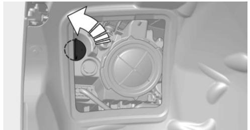
3. Press the bulb gently into the socket, turn counterclockwise and remove.
