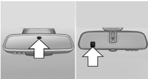
Photocells are used for control:
