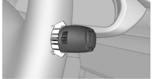
Turn the thumbwheel to adjust the frequency or sensitivity of the rain sensor.
