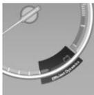
The kinetic energy of the vehicle is converted to electrical energy while Coasting. The vehicle battery is partially charged and fuel consumption can be reduced.
