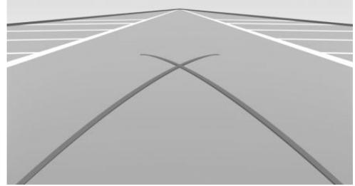
Turning circle lines can only be superimposed on the rearview camera image together with pathway lines.
