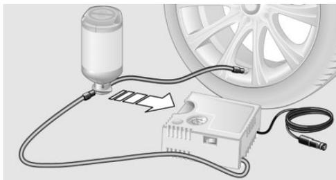
5. Screw the filling hose of the sealant container onto the tire valve of the nonworking wheel.
