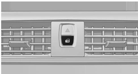
Pressing the central locking system button locks or unlocks the vehicle with the doors closed.
