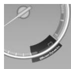
In coasting overrun mode the kinetic energy of the vehicle is converted to electrical energy. The vehicle battery is partially charged and fuel consumption can be reduced.
