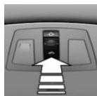
Press the switch up and hold it until initialization is complete.
