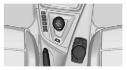
Press the button repeatedly until the desired driving program is displayed in the instrument cluster.
