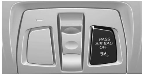
The indicator light for the front-seat passenger airbags indicates the operating state of the front-seat passenger airbags.
