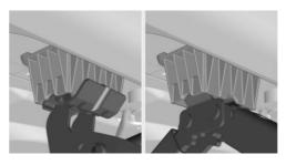
3. Extend the vehicle jack by turning the vehicle jack crank or lever clockwise.
