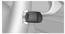
Turn the thumbwheel on the wiper lever.
