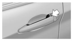
Touch the surface on the door handle of the driver's or front passenger door with your finger for approx. 1 second without grasping the door handle. This corresponds to pressing the button 🔇 on the vehicle key.
