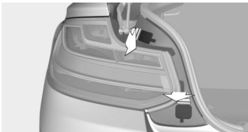
3. With the handle of the screwdriver from the onboard vehicle tool kit, loosen and remove the nuts on the two fasteners. Make sure that the nuts do not drop into the bumper area. In addition to the two outer fasteners, there is another inner fastener.
