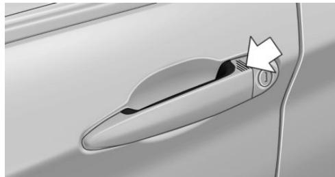
Touch the surface on the door handle of the driver's or front passenger door, arrow, with your finger and hold it there without grasping the door handle.
