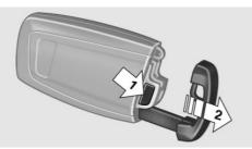
Press the button, arrow 1, and pull out the integrated key, arrow 2.
