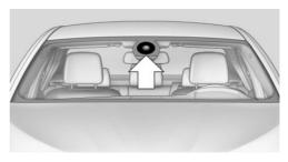
The camera is installed near the interior mirror. Keep the windshield in front of the interior mirror clean and clear.
