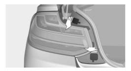
With the handle of the screwdriver from the onboard vehicle tool kit, loosen and remove the nuts on the two fasteners. Make sure that the nuts do not drop into the bumper area. In addition to the two outer fasteners, there is another inner fastener.
