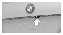
The camera lens is located in the handle of the tailgate.
