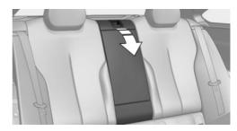
Reach into the recess and pull the center section forward.
