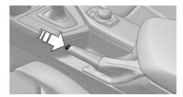
Raise lever slightly, press the button and guide the lever down.
