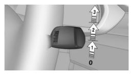
Press the lever up once from its standard position, arrow 1.
