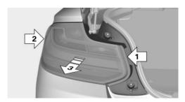
5. Remove the plug from the bulb holder.
