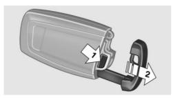
Press the button, arrow 1, and pull out the integrated key, arrow 2.
