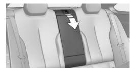
Press the switch and pull the center section forward.
