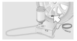
6. With the compressor switched off, insert the plug into the power socket inside the vehicle.
