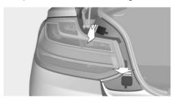
With the handle of the screwdriver from the onboard vehicle tool kit, loosen and remove the nuts on the two fasteners. Make sure that the nuts do not drop into the bumper area. In addition to the two outer fasteners, there is another inner fastener.
