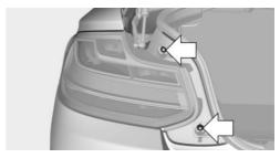
4. Hold the grip rail in one hand, arrow 1, and brace against the outside with your other hand, arrow 2. Carefully pry out the tail light, arrow 3, until the rubber mount releases from the inner fastener.
