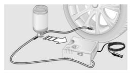
Remove the valve cap from the tire valve and screw the filling hose of the sealant container onto the tire valve of the nonworking wheel.
