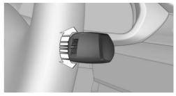
Turn the thumbwheel on the wiper lever.
