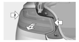
5. Remove the plug from the bulb holder.
