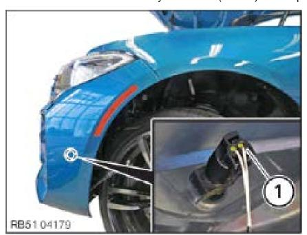
\*\*\* a word of warning here – don't start the car with this removed or it will set off a "check engine light" .....ask me how I know! The plug slides off by pushing in a typical clip.
