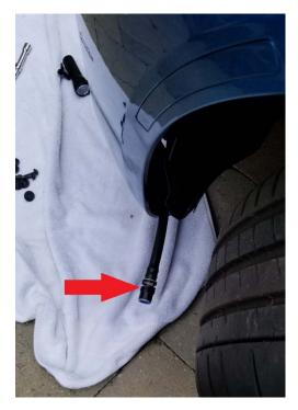
Turn the ends of the washer units (where the hoses connect – they can swivel) up so they clear when you remove the bumper.
