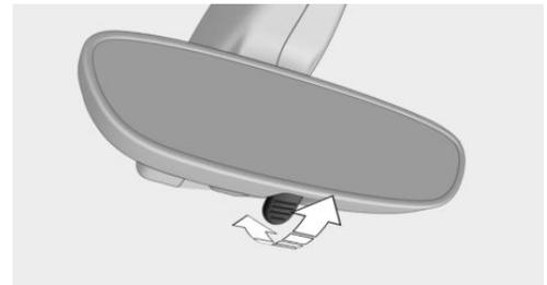
To reduce the blinding effect of the interior mirror, flip the lever forward.
