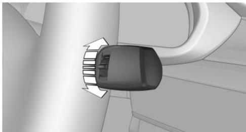
Turn the thumbwheel on the wiper lever.
