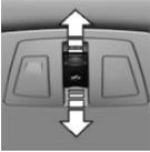
2. Push the switch forward again past the resistance point and hold until the glass sunroof closes without jam protection. Make sure that the closing area is clear.
