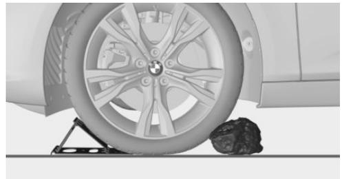
Place chocks or other suitable objects, for example a rock, in front of and behind the wheel that is diagonally opposite to the wheel that you wish to change.
