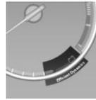
In coasting overrun mode the kinetic energy of the vehicle is converted to electrical energy. The vehicle battery is partially charged and fuel consumption can be reduced.
