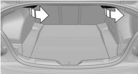
2. The unlocked rear seat backrest moves forward slightly.
