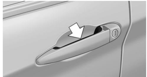
Grasp the door handle on the driver's or front passenger door completely.
