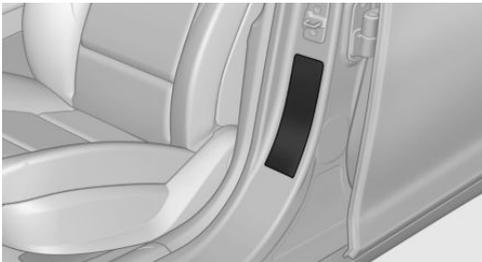
These tire inflation pressure values can also be found on the tire inflation pressure label on the driver's door pillar.
