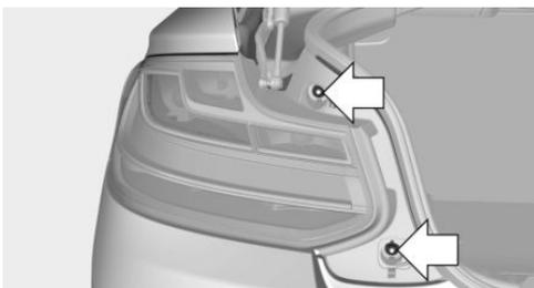
4. Hold the grip rail in one hand, arrow 1, and brace against the outside with your other hand, arrow 2. Carefully pry out the tail light, arrow 3, until the rubber mount releases from the inner fastener.
