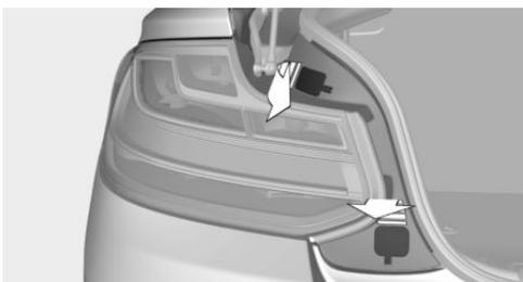
3. With the handle of the screwdriver from the onboard vehicle tool kit, loosen and remove the nuts on the two fasteners. Make sure that the nuts do not drop into the bumper area. In addition to the two outer fasteners, there is another inner fastener.
