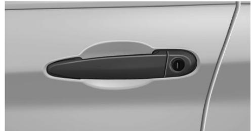
Unlock or lock the driver's door via the door lock using the integrated key, refer to page 34. The other doors must be unlocked or locked from the inside.
