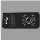
An external audio device, for example, an MP3 player, can be connected via the AUX-IN port or the USB audio interface in the center armrest.
