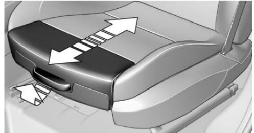
Pull the lever at the front of the seat and adjust the thigh support.
