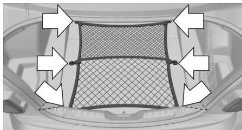
Hook the floor net into the fittings in the cargo area floor.
