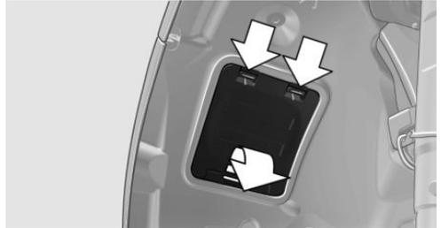
2. If necessary, pull the inside trim of the wheel house slightly inward. Turn the bulb socket counterclockwise and remove.
