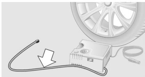
3. Screw the connection hose onto the connector of the sealant container.
