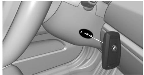
1. Hold the remote control with its back against the marked area on the steering column.
