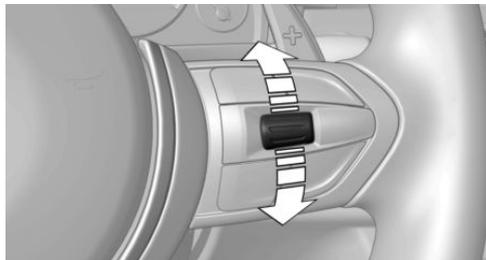
On the right side of the steering wheel, turn the thumbwheel to activate the corresponding list.
