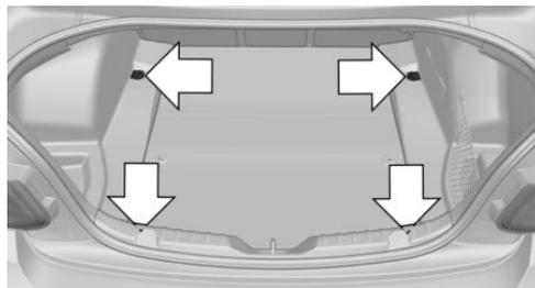
To secure the cargo there are two or four lashing eyes in the cargo area.
